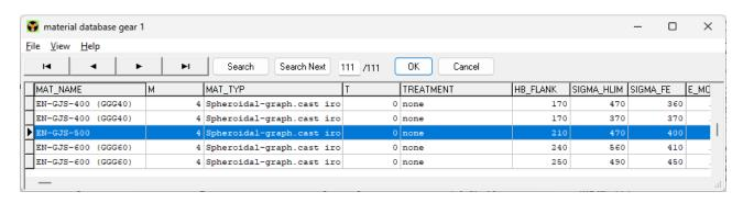
GJS-500 has been added to the gear material database. Its strength values are between GJS-400 and GJS-600.
