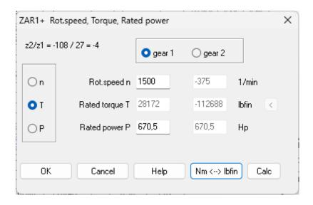
When switching to imperial settings, the text for entering the coefficients changes. The face width factor b/mn in mm is equal to b[in] \* DP[1/in].
